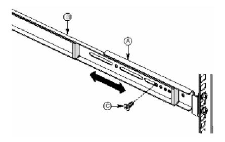
Figure 39: Attaching Rail Assembly to Rear Bracket
